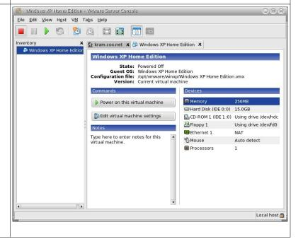
Clicking on the RUN button starts the Vmware virtual machine. It is just like booting a real X86 machine, complete with a virtual BIOS.
