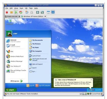
Install the VMWare tools into the guest OS. It is quite easy and it will greatly enhance the speed and efficiency of the OS running in the virtual machine. It will install some MS-Windows drivers, one of which will allow you share files with the host OS (Linux).
